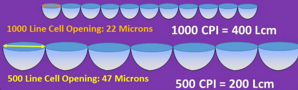
Figure 1: The linescreen is defined by how many cells are present per linear inch on the roll (lpi).
