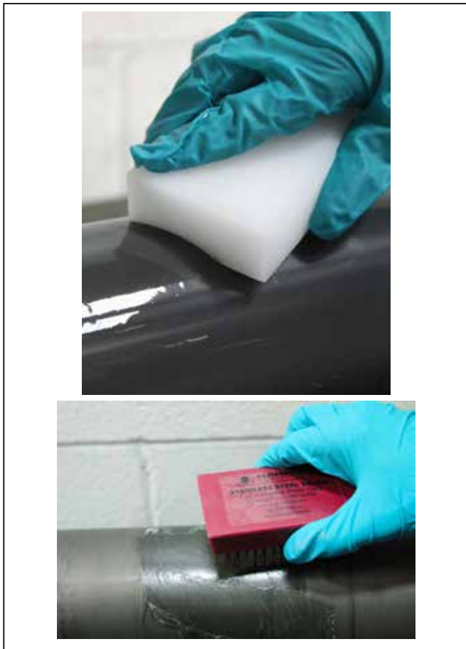
Using the proper cleaning apparatuses and solutions can make a world of difference in maintaining an anilox roll.
